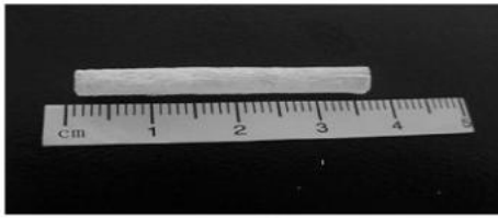
图1 类人胶原蛋白-透明质酸血管支架的外部形态 Fig. 1 Appearance of human-like collagen-hyaluronic acid blood vessel graft.
