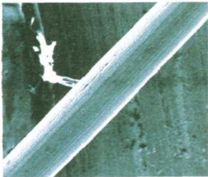
图 2 浸泡处理后的镍钛合金丝扫描电镜照片 (×100 倍) Fig. 2 Electron microscopic picture of Ni-Ti alloy after treatment (×100)
