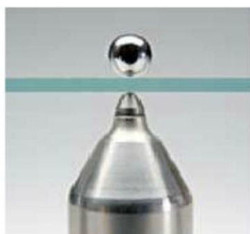
Reference balls with a specially coated finish and dimensional precision to obtain maximum reproducibility of readings.
